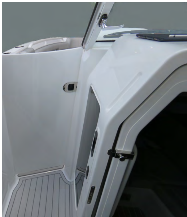
Cabin Door Latched In Open Position
