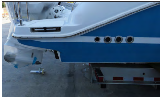
Hull Side Scupper Drain Thru-Hulls
