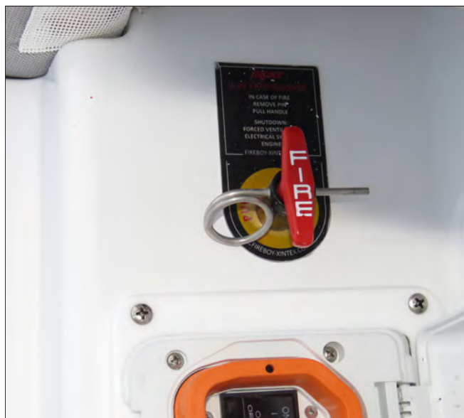
Manual Pull Station In Aft Cockpit
