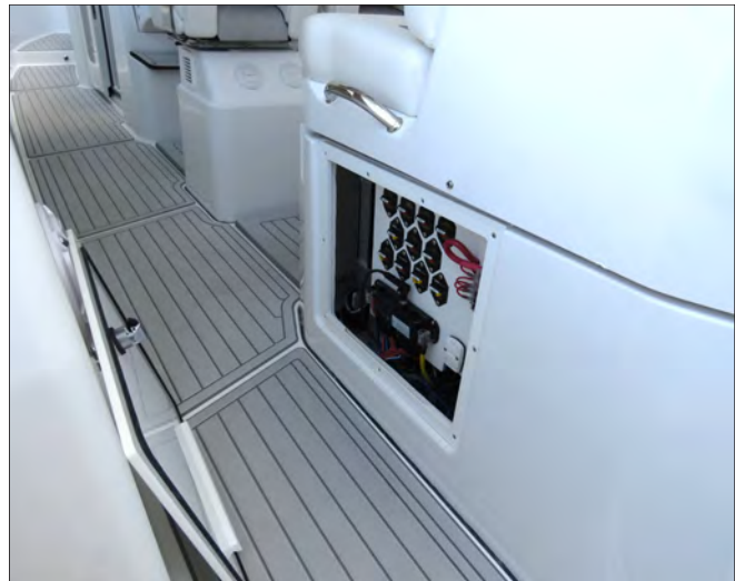
Removable Access Door On Port Side Of Mezzanine
