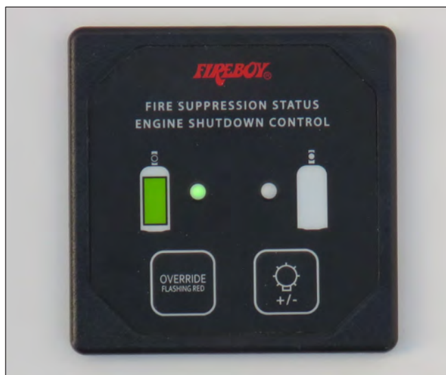
Fire Extinguisher Panel In Helm
