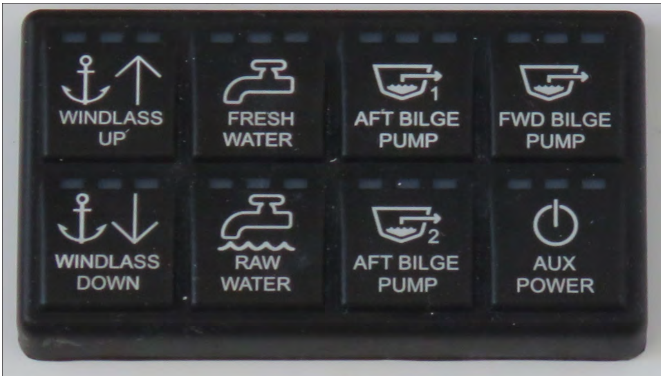
Starboard Helm Switch Panel
