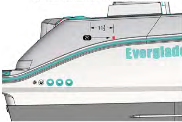
AFT STARBOARD SLING LOCATION, MIRROR FOR PORT
