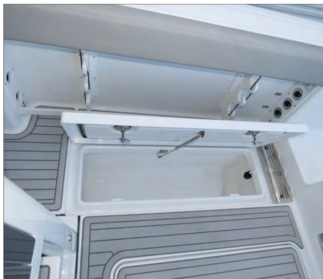
Aft Below Deck Fishbox
