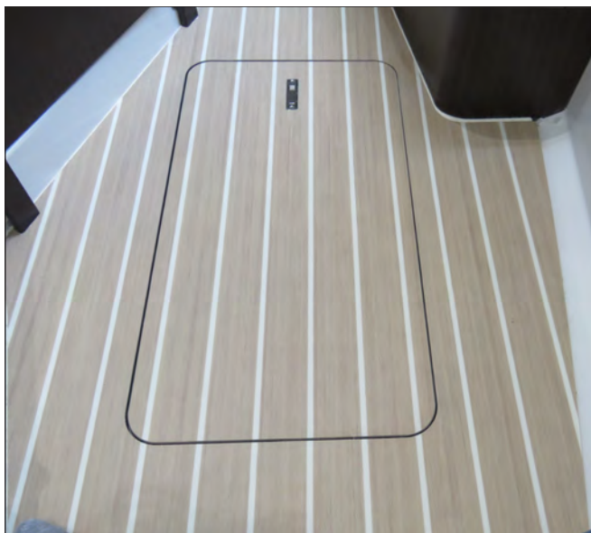
Cabin Sump System Access Hatch
