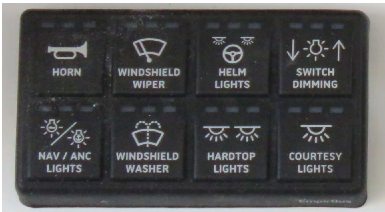
Port Helm Switch Panel
